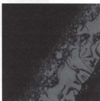
Sample 5f : nematic from isotropic liquid at 250°C, on cooling
