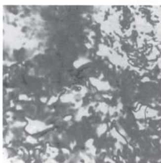
Sample 5d : nematic texture at 220°C, on heating
