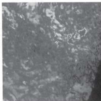
Sample 6g : nematic mesophase at 250°C (after re-disordering phenomena) on heating
